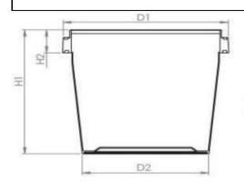
D1 = 70,5 ± 1 mm D2 = 54.0 ± 1 mm H1= 65.0 ± 0.5 mm H2 = 12.0 ± 0.5 mm
