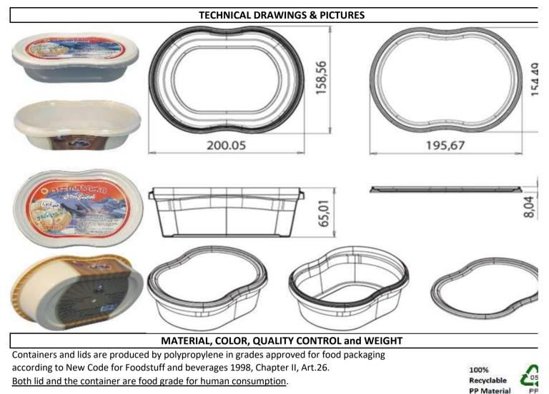
DÖK1500 container and lid can be produced with all colors as per the demand of the customer. Production is certificated according to EN ISO 9001:2000. Container: 51 gr (±1) Lid: 29 gr (±1) Volume: 1500 ml
