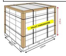
**Box Dimensions (tub)** 40\*60\*48 cm (w \* I \* h) Box Dimensions (lid) 40\*60\*48 cm (w \* I \* h) Boxes per Pallet 20 **Quantity per Pallet** 34.800 pieces (Tub) Quantity per Pallet 30.800 pieces (Lid) Quantity per Truck 539.000 sets (Set = Body + Lid)Quantity per 40'HC Container 392.000 sets (Set = Body + Lid)Quantity per 20'DC Container 180.000 sets (Set = Body + Lid)
